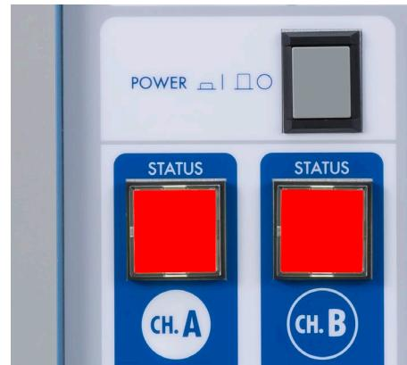
② After about 12 seconds, the buzzer sounds and the touch screen displays the start screen. (The mode selected for CH.A and CH.B changes based on usage history.)
