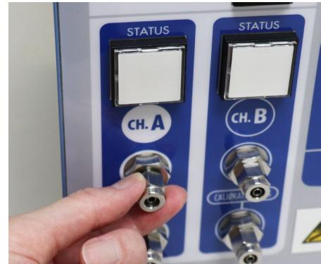
② Insert the FEP tube into the nipple.
