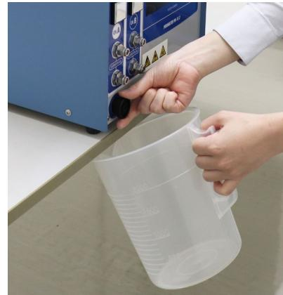
④ After draining, close WATER DRAIN.
