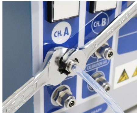
④ Check that the FEP tube does not come out easily by pulling gently.
