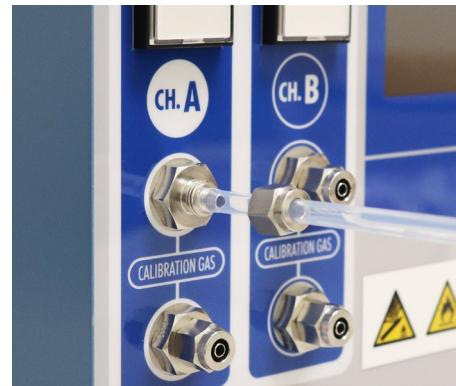
③ Tighten the nut to hold the FEP tube. (Example of CH.A)
