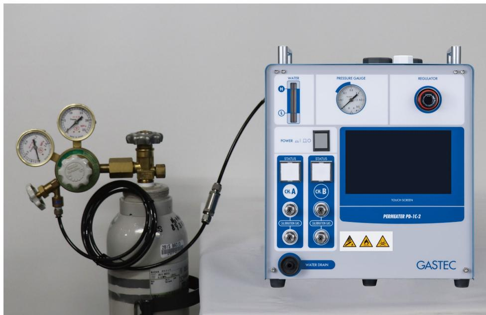
\*An example of connection with high-pressure air cylinder
