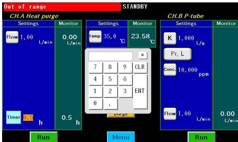
Touch and hold "Run" to start Heat purge. The status on the screen will show "HEAT RUNNING" and the STATUS lamp will illuminate green. (When the temperature setting is 35.1°C or higher, it will flash slowly.)
