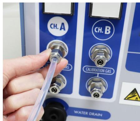
The spanner for holding down the nut on the main unit (17mm) and the spanner for tightening the tube fixing nut (12mm) are not supplied with this product.
