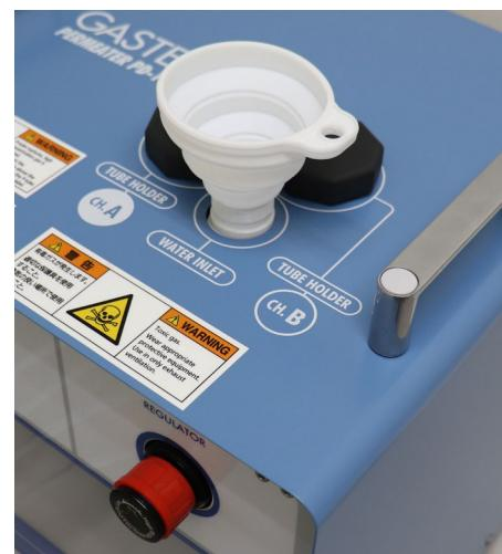
⑦ Make sure the inlet you are pouring water is WATER INLET (constant temperature tank inlet). Watch the WATER (water level gauge) gauge and pour water between levels H and L. Overflow may occur due to slow response of the WATER gauge. If level L is exceeded, pour water slowly.
