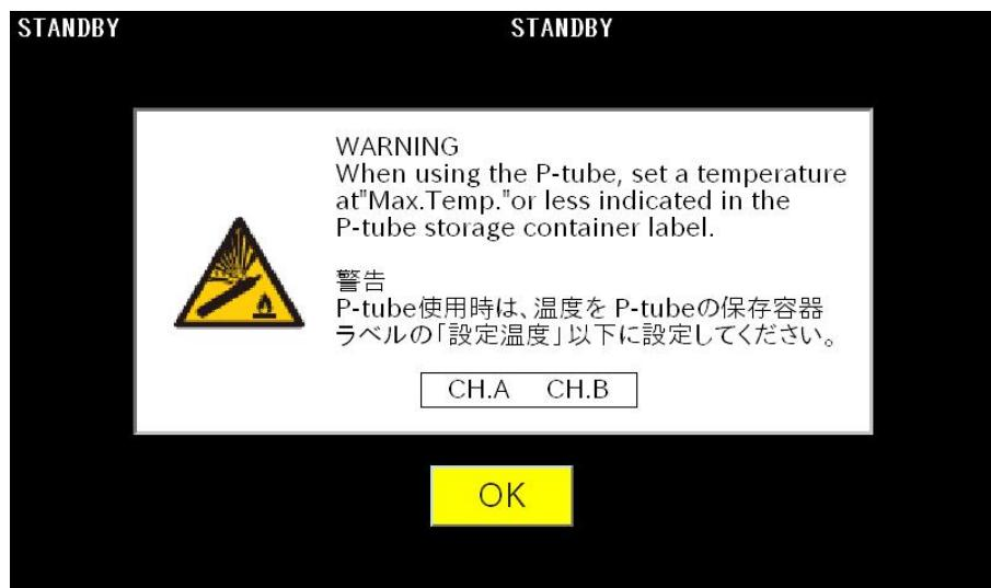
(Confirmation screen when both CH.A and CH.B are in P-tube mode)
