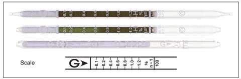
When used, these tubes are to be connected. This detector tube is calibrated with Propane.
