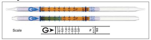
**Performance** The minimum scale value (0.05%) is not printed on the tube, but only the scale line is printed.
