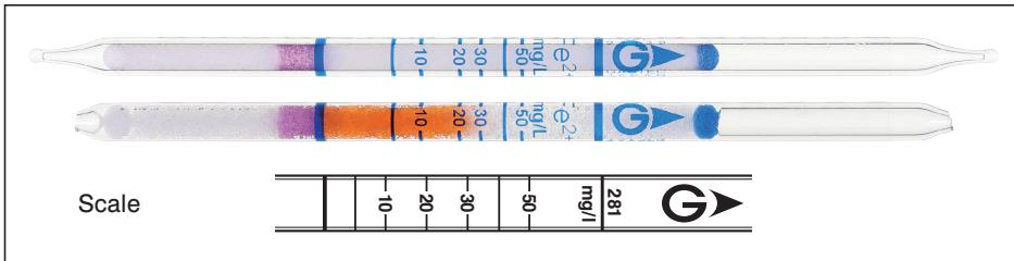
**Performance** The minimum scale value (5mg/L) is not printed on the tube, but only the scale line is printed.
