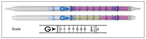
**Performance** The minimum scale value (1ppm) is not printed on the tube, but only the scale line is printed.
