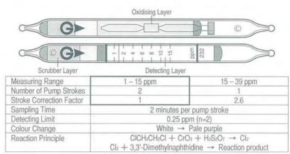
Coefficient of Variation : 15% (for 1 to 4 ppm), 10% (for 4 to 15 ppm) \*\*Shelf Life : Please refer to the validity date printed on the tube box. \*\*Store the tubes at  $10^{\circ}C$  ( $50^{\circ}F$ ) or below in the refrigerator.
